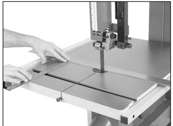
Figure 34. Measuring for miter slot to be parallel with blade.
