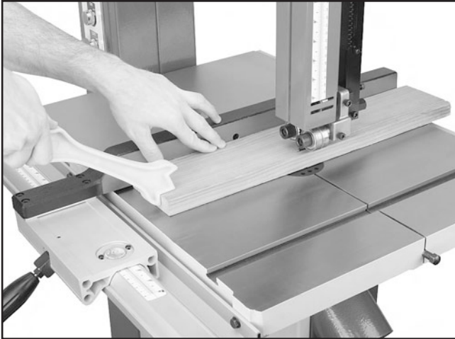
Figure 43. Ripping with a push stick.
