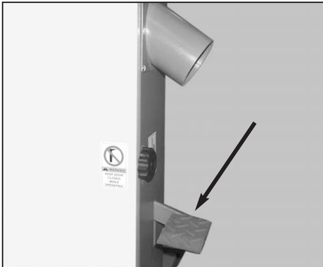
Figure 21. The foot brake is located below the dust collection port.
