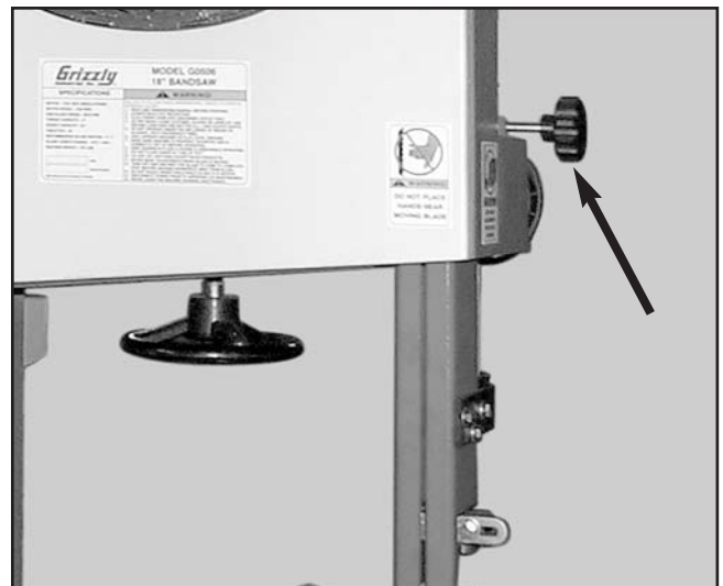
Figure 9. Guide post lock knob.
