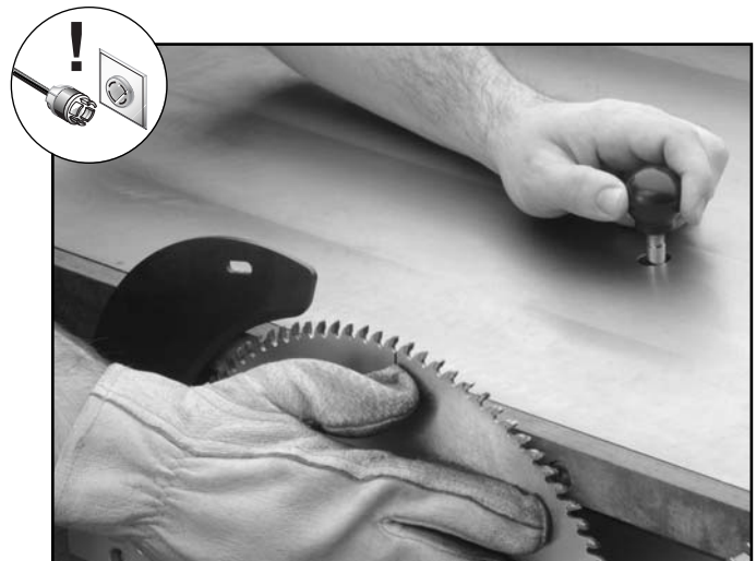
Figure 81. Locking main blade with the lock tool.
