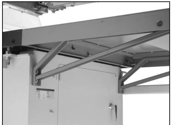
Figure 41. Large extension table installed.
