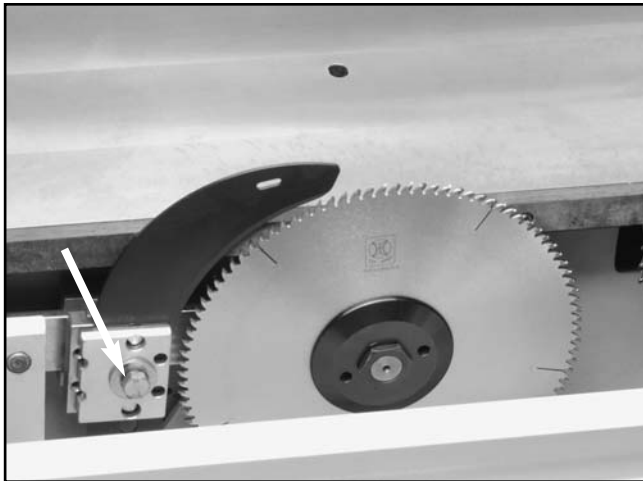
Figure 92. Riving knife securing bolt.
