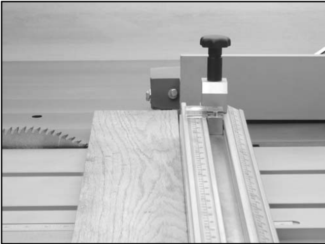
Figure 73. Correct rip fence position when performing crosscutting operations.
