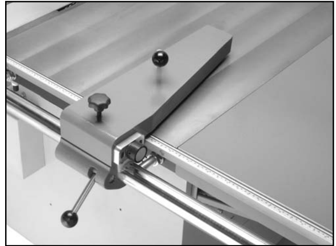
Figure 43. Installed clamp assembly.
