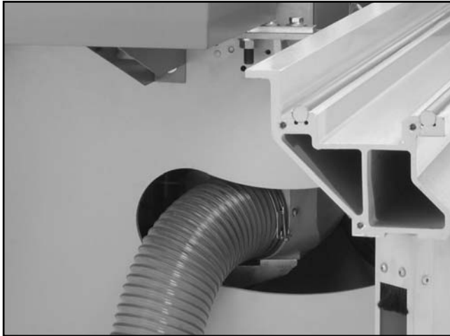
Figure 59. 5" dust port location.
