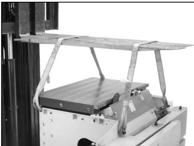
Figure 19. Lifting the saw base unit.
