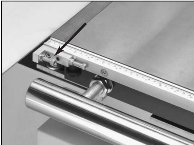
Figure 56. Rip fence stop bolts
