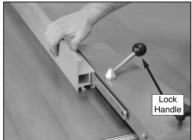
Figure 44. Installing aluminum fence to clamping assembly in upward position.
