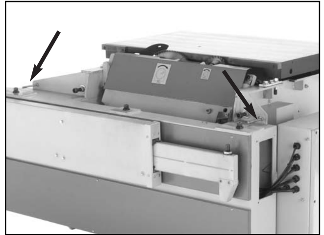
Figure 26. Parallel adjustment bolts.
