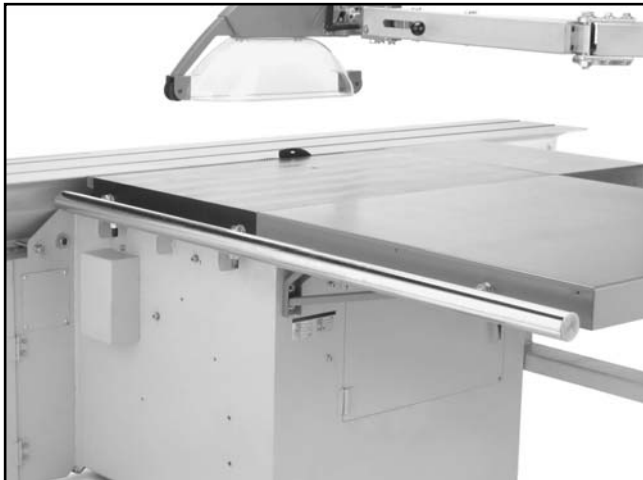
Figure 42. Fence rail installed.
