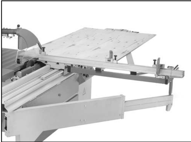
Figure 65. Rip cutting setup with the sliding table.
