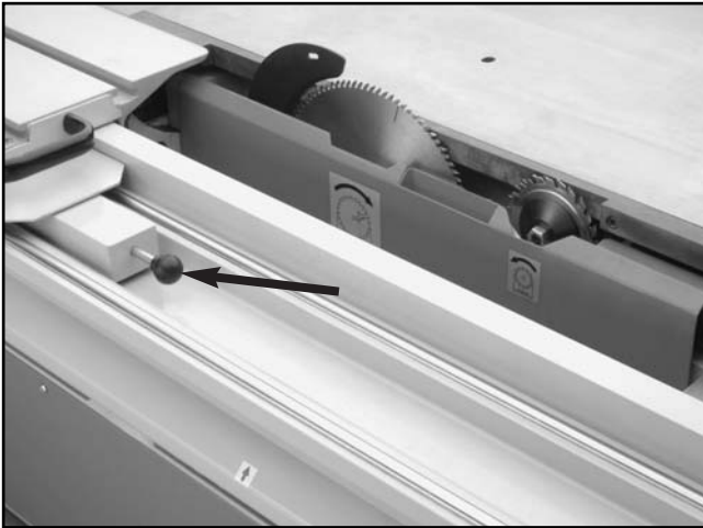
Figure 87. Sliding table release knob.
