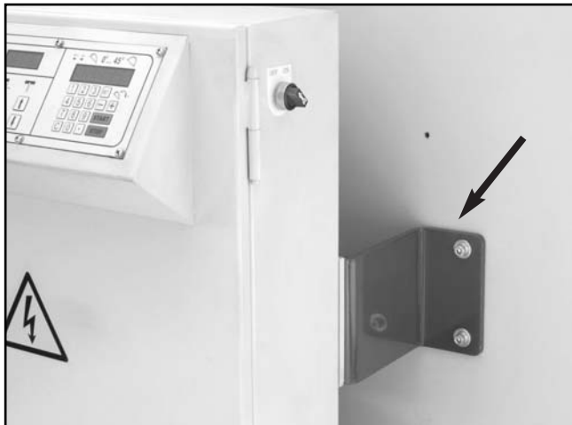
Figure 21. Control panel shipping brace.
