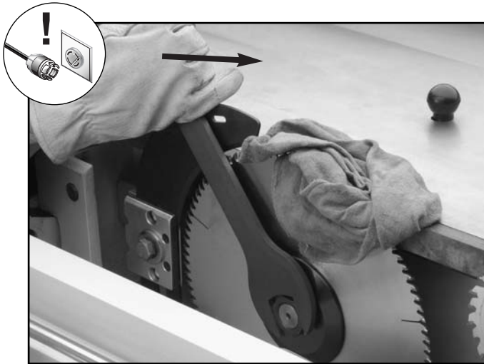
Figure 82. Removing arbor nut to change blade.
