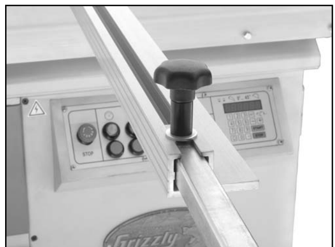
Figure 79. Miter fence slide installation for cut lengths between 45" and 86½".
