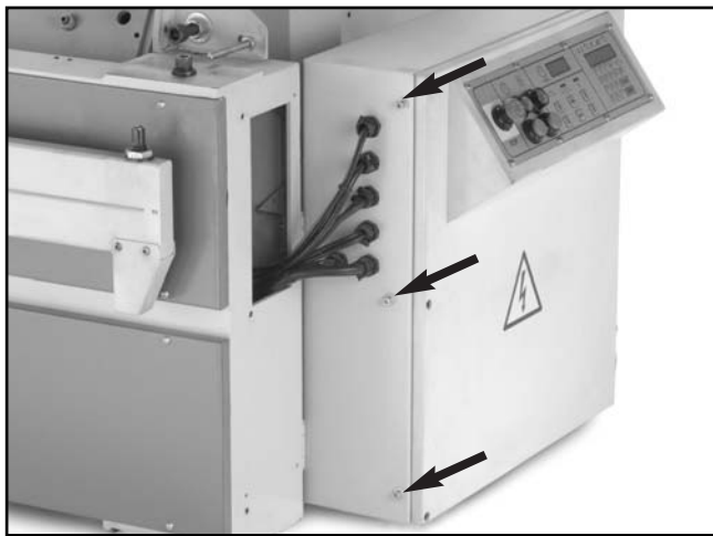
Figure 22. Control panel face and side cap screws.
