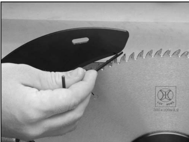
Figure 85. Checking riving knife distance from blade tip with 3mm hex wrench.
