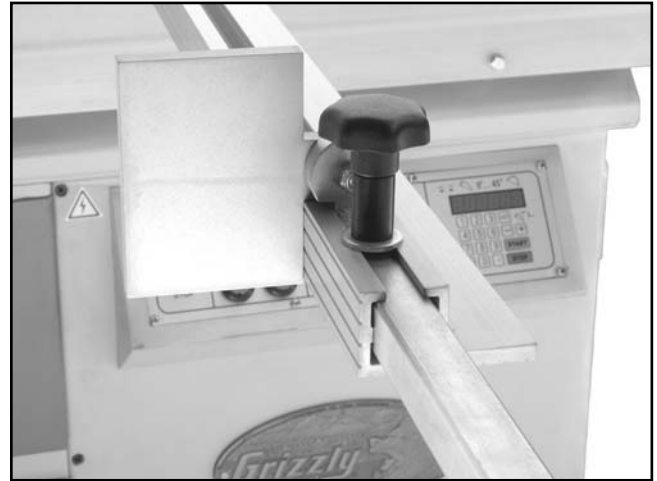
Figure 78. Miter fence slide installation for cut lengths between 9½" and 45".
