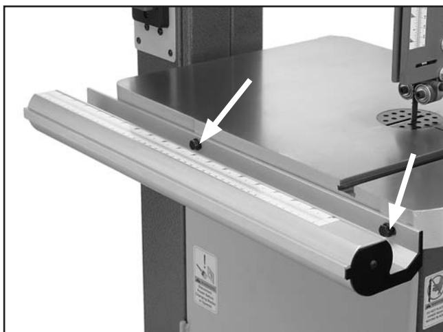
Figure 16. Installed front rail.
