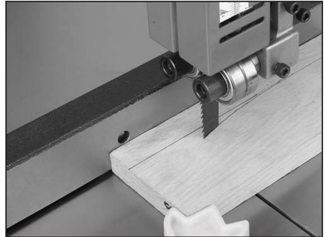
Figure 62. Blade leading away from line of cut.
