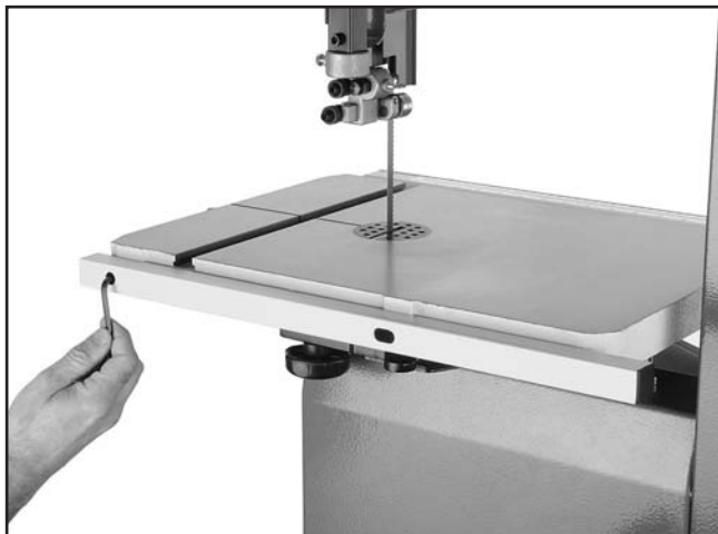
Figure 15. Rear rail installed.
