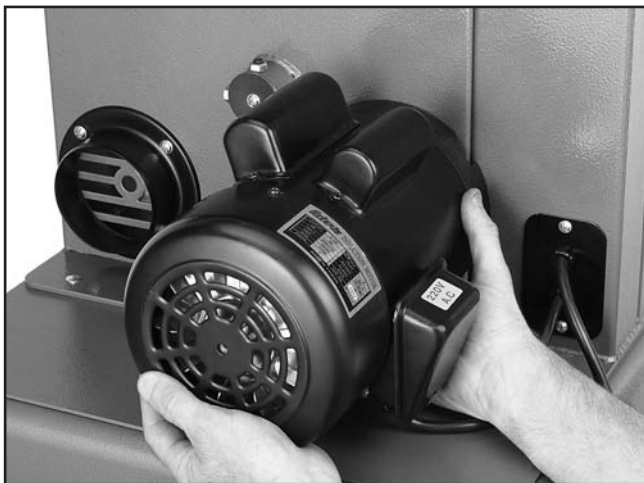
Figure 12. Installing motor (outside view).
