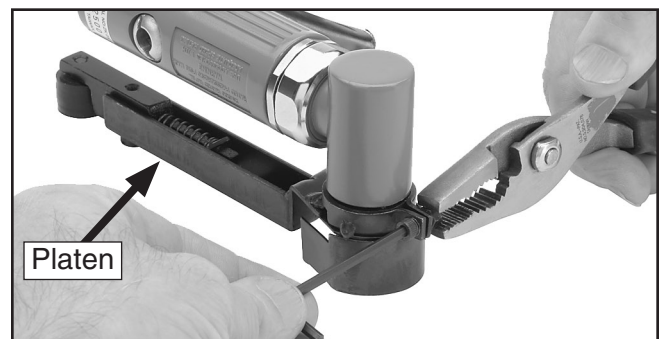
Figure 2. Loosening cap screw and hex nut.
