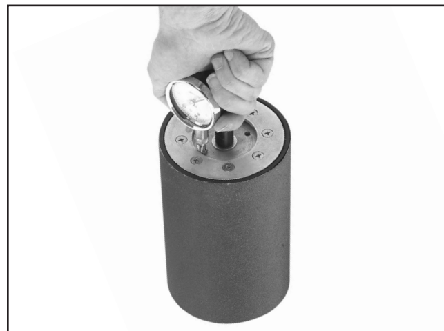
Figure 12. Checking sanding drum air pressure.
