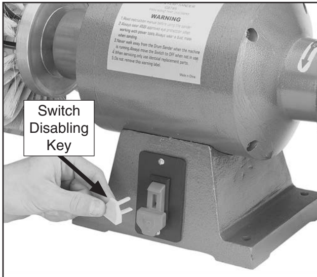
Figure 14. Removing the ON/OFF switch disabling key.
