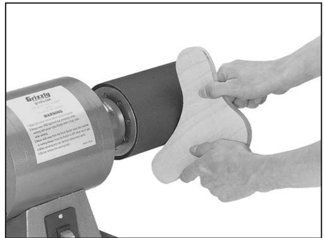
Figure 1. Typical drum sanding operation.
