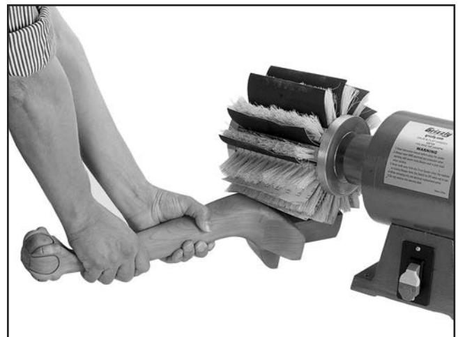
Figure 2. Typical flap sanding operation.
