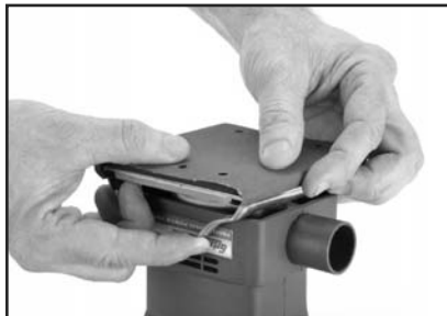
Figure 4. Attaching sandpaper on the opposite side
