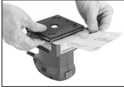
Figure 3. Attaching sandpaper on one side.
