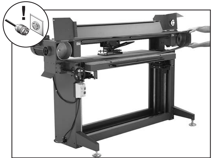
Figure 37. Installing new belt.
