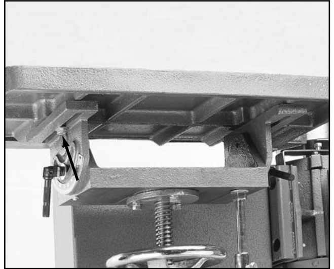
Figure 10. Attaching the working table.
