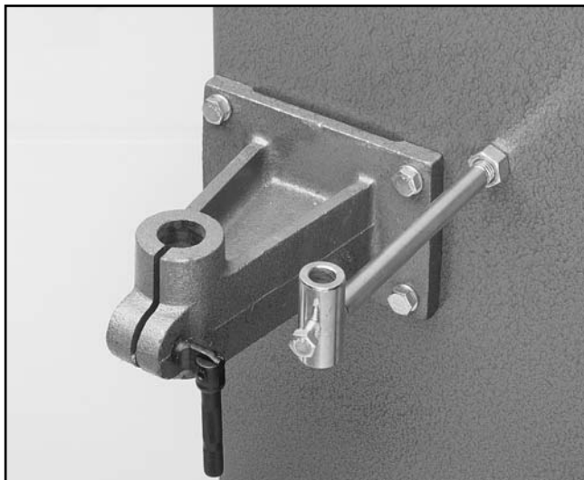
Figure 5. Installing the horizontal brace.
