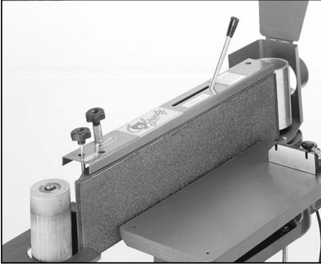
Figure 16. Sander ready for belt installation.
