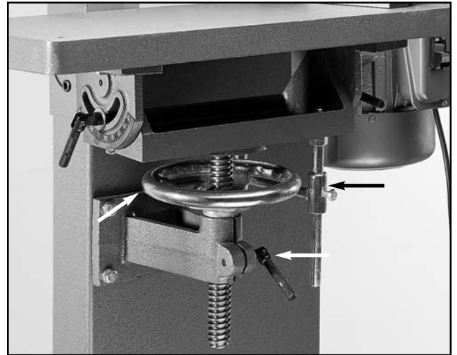
Figure 22. Table height adjustment.
