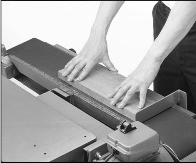
Figure 28. Typical face sanding method.
