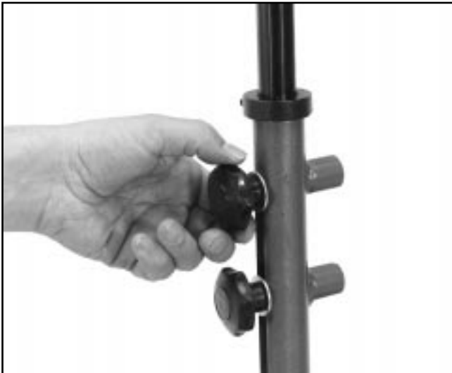
Figure 9. Tightening sanding arm knobs.
