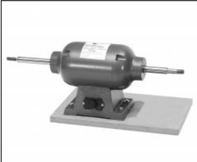
Figure 4. Motor secured to base.
