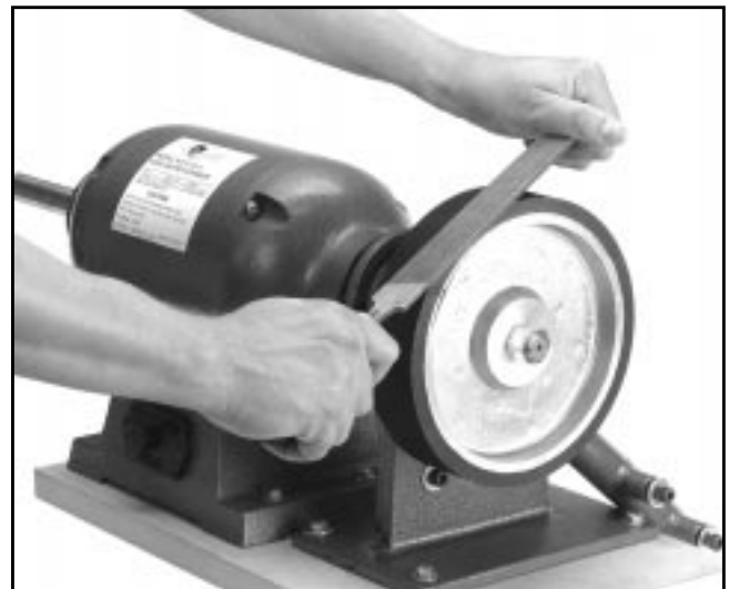
Figure 15. Relieving edges of drive wheel.
