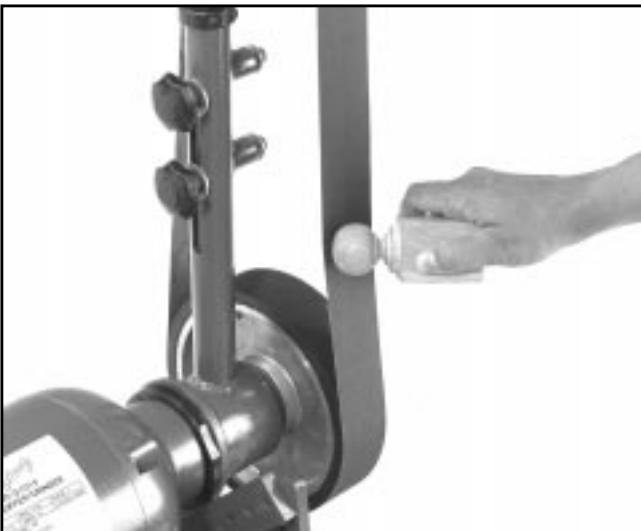
Figure 18. Contour sanding, shoe removed.
