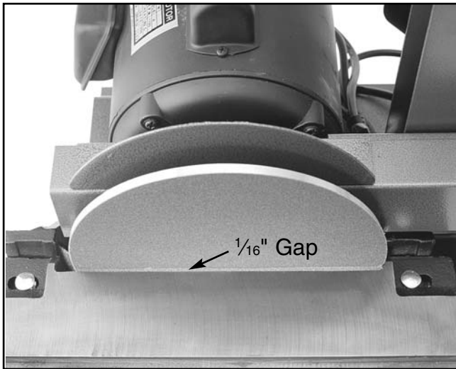
Figure 13. Table aligned with sanding disc.
