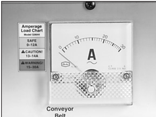
Figure 23. Amp load meter.
