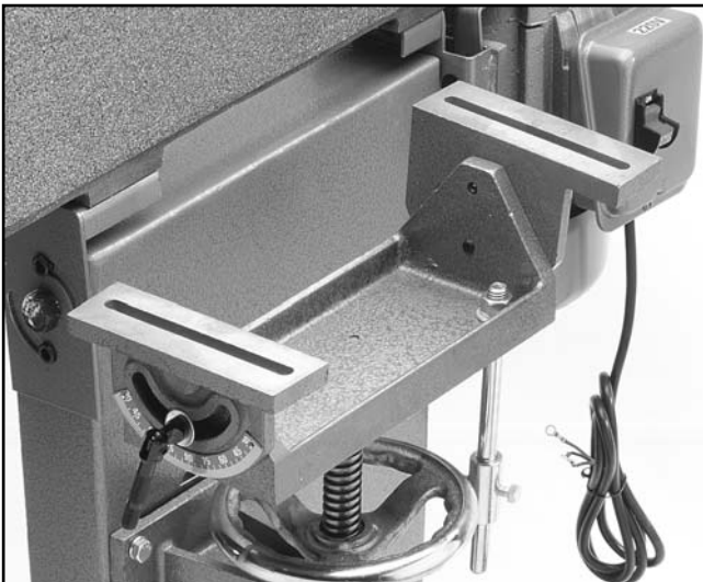
Figure 9. Table trunnions installed.
