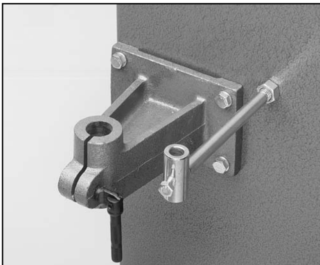
Figure 5. Installing the horizontal brace.
