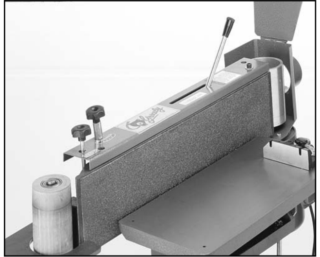
Figure 17. Sander ready for belt installation.
