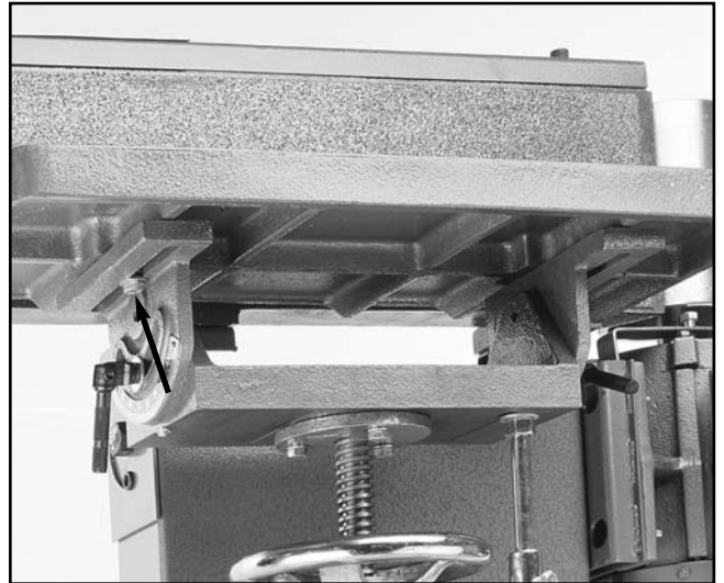
Figure 10. Attaching the working table.
