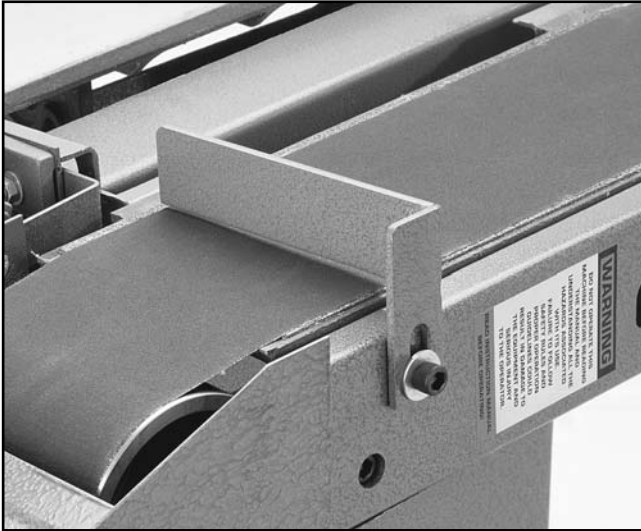
Figure 16. Back stop properly installed.
