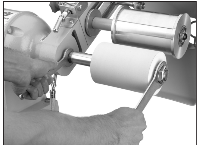
Figure 11. Replacing the sanding drums.
