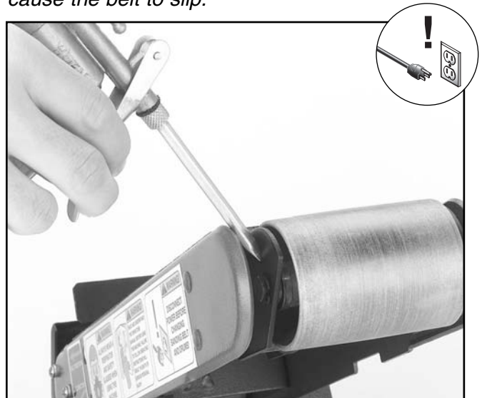
Figure 25. Lubricating the sleeve bearings.
