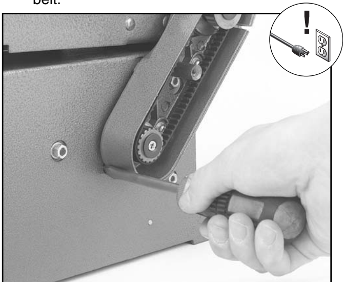
Figure 24. Tensioning the drive belt.
