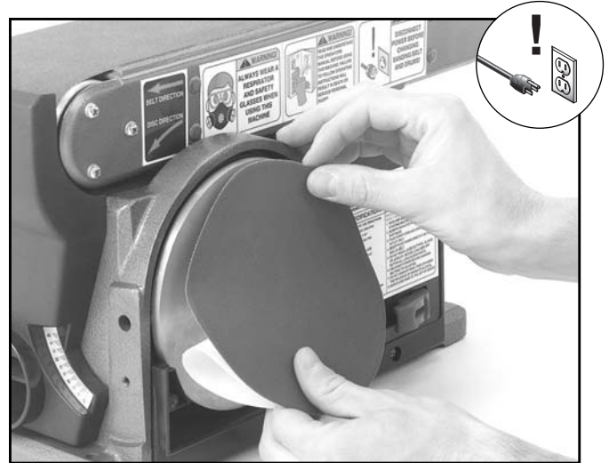
Figure 8. Center the sandpaper on the disc.
