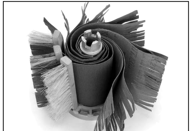
Figure 25. Re-assembling the flap sander.
