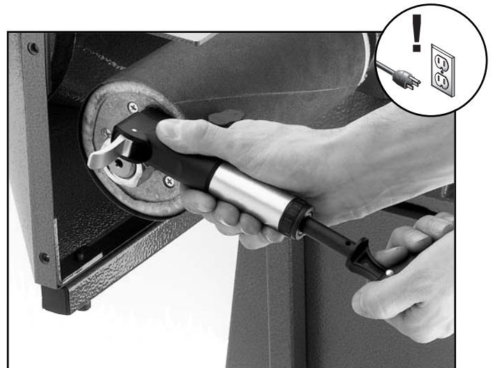
Figure 14. Inflating the sanding drum.
