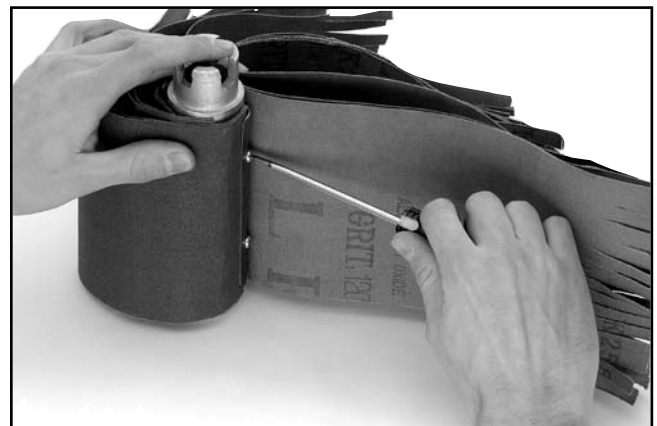
Figure 26. Removing sandpaper clamps.
