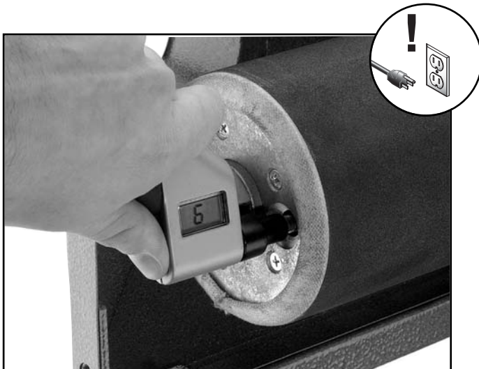
Figure 20. Checking air pressure.
