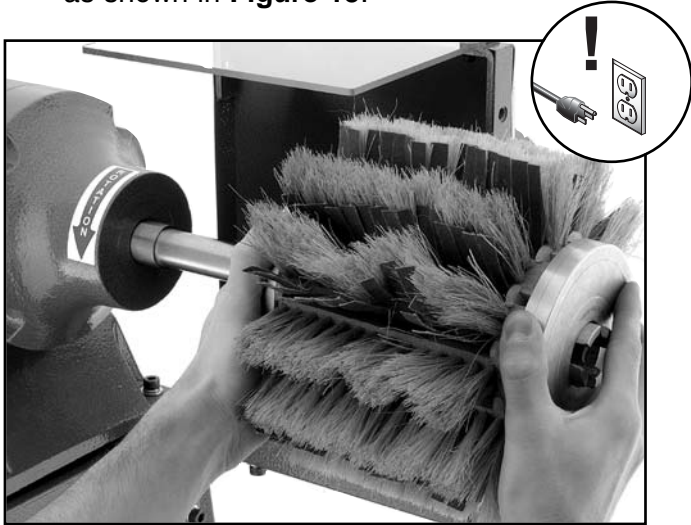
Figure 15. Sliding the flap sander onto the arbor.
