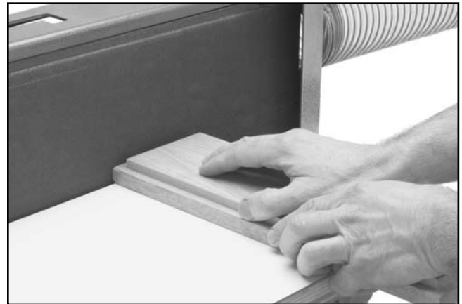
Figure 24. Typical end sanding operation.
