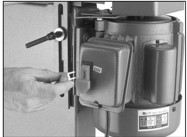
Figure 21. Safety key removed from switch.
