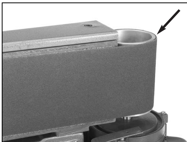
Figure 11. Sanding belt even with top of main roller.
