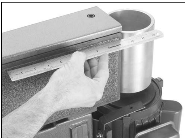
Figure 41. Checking top of platen-to-roller.
