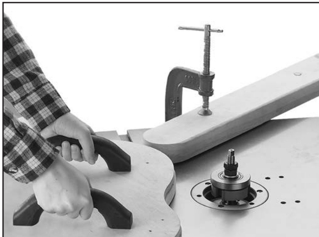
Figure 22. Generic picture of using a jig with a starting block (guard removed for photo clarity).
