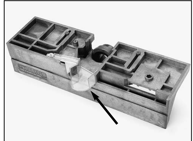
Figure 12. Correctly installed guard.
