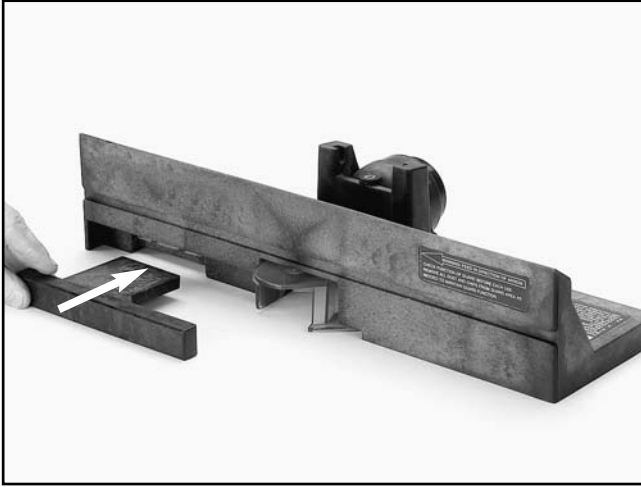
Figure 13. Installing the pocket jointing fence.
