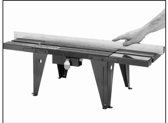
Figure 6. Using a straightedge to ensure the working surfaces are flush.
