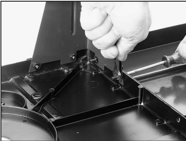
Figure 5. Securing a leg to the main table.
