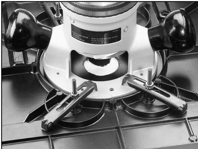
Figure 10. Correctly clamped router.
