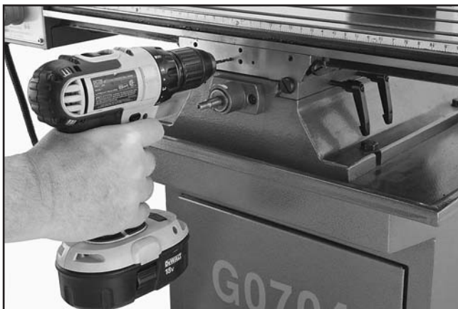
Figure 14. Drilling holes for limit switch assembly.
