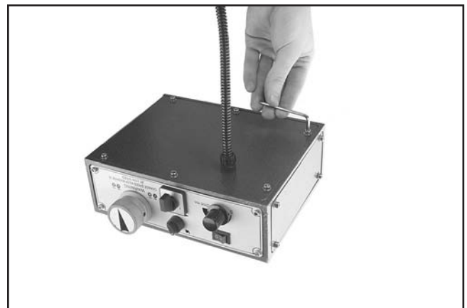
Figure 5. Removing bottom cover.
