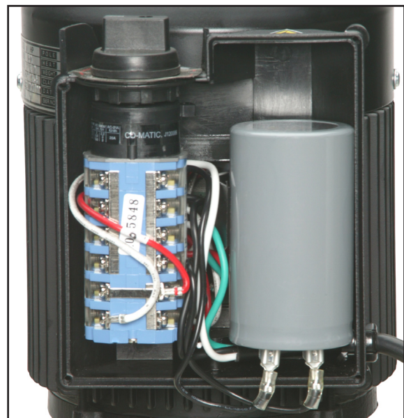
Figure 19. Motor switch and capacitor (front view).
