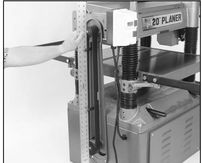
Figure 28. Pulley alignment procedure.
