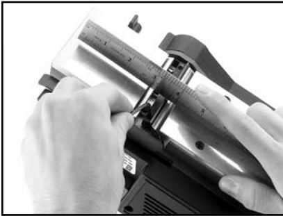
Figure 10. Setting cutter height.
