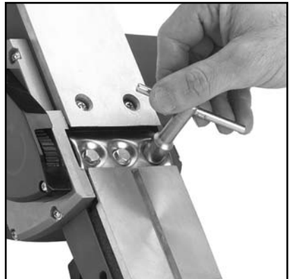
Figure 3. Removing Blade Holder bolts.
