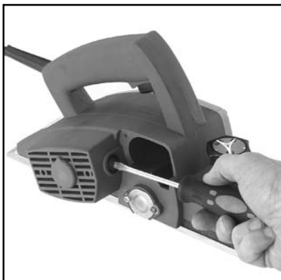
Fig 10. Replacing motor brushes.
