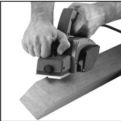
Fig 7. Cutting a chamfer.
