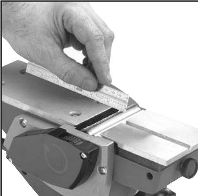
Figure 2. Checking Blade height.
