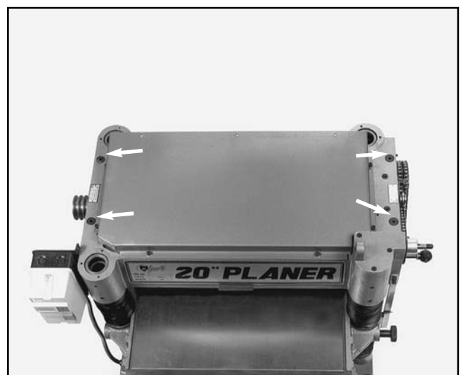
Figure 41. Feed roller lubrication points.
