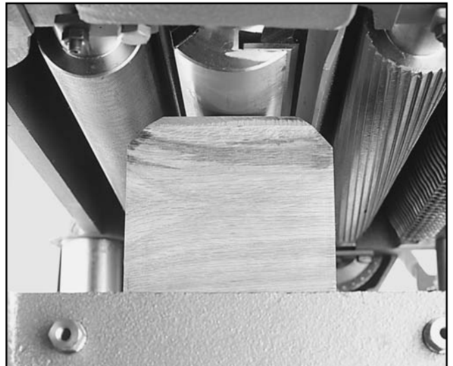
Figure 12. Guide block indicates parallelism.
