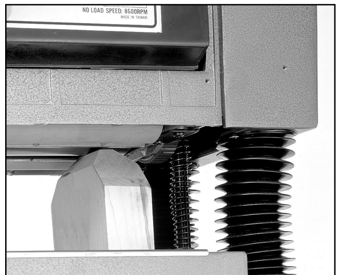
Figure 8. Using gauge to check cutterhead.
