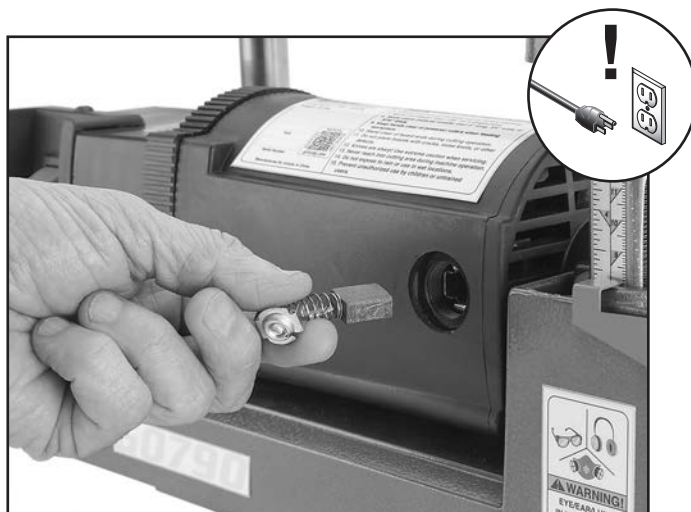
Figure 31. Brush holder location. A second brush is located on other side of motor.
