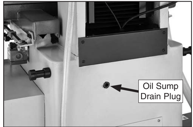
Figure 46. Location of oil sump drain plug.
