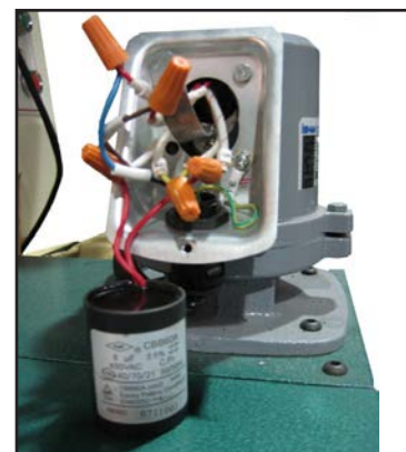
Figure 56. Coolant motor wiring (220V).
