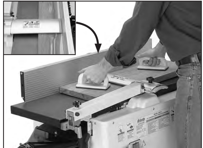
Figure 33. Surface planing board less than 3" thick.
