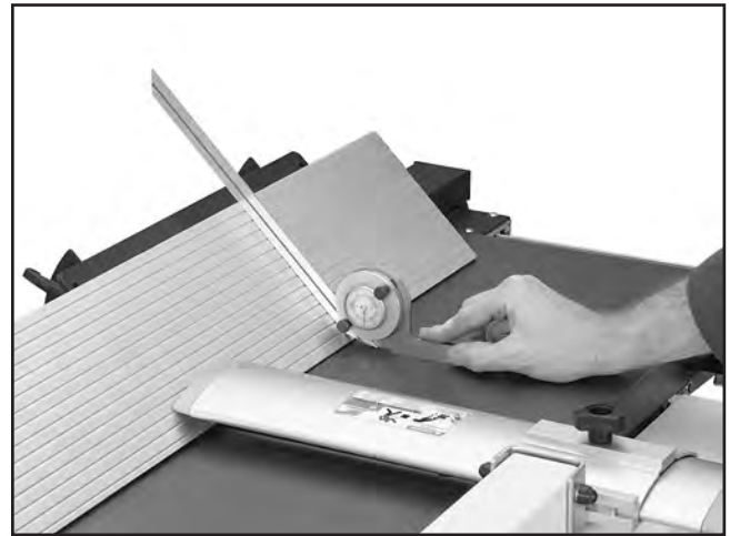
Figure 72. Adjusting fence 45° outward.
