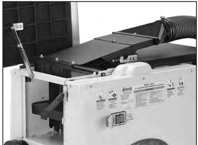
Figure 15. Dust hose attached to dust port setup for planer operations.
