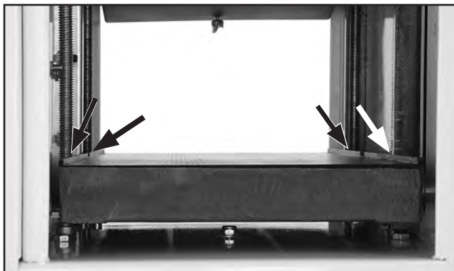
Figure 51. Leadscrew-planer table lubrication locations.
