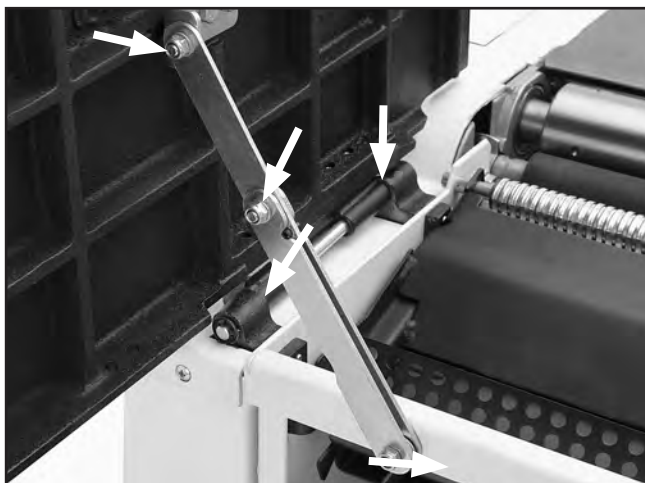
Figure 54. Outfeed table lubrication points.
