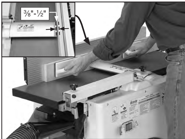
Figure 35. Edge jointing operation.
