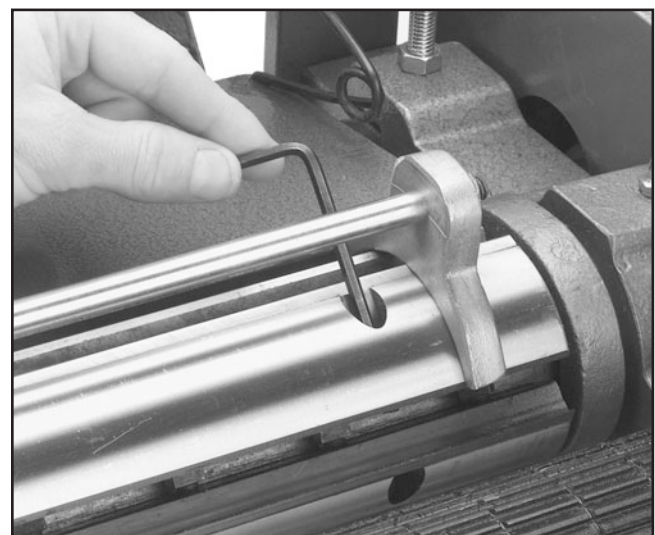
Figure 8. Adjusting knife height.
