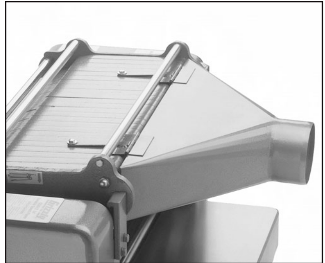
Figure 4. Dust hood installed.
