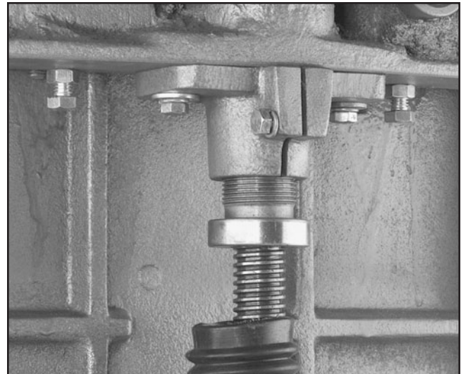
Figure 12. Column adjustment flange underneath table.
