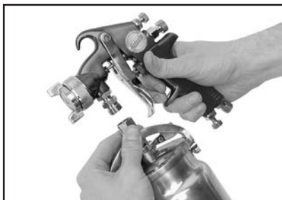
Figure 2. Attaching the spray gun body to the fluid cup.
