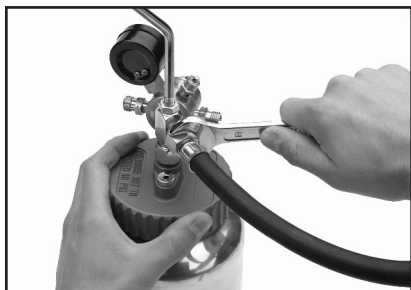
Figure 3. Installing fluid hose.
