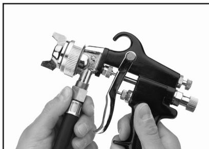
Figure 4. Attaching fluid hose to spray gun.
