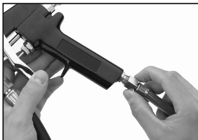
Figure 6. Attaching hose to spray gun.
