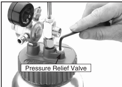
Figure 20. Pressure relief valve.
