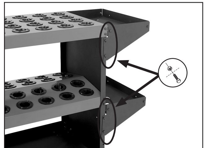
Figure 10. Side shelf assemblies installed.
