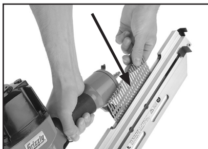
Figure 4. Loading nails into magazine.
