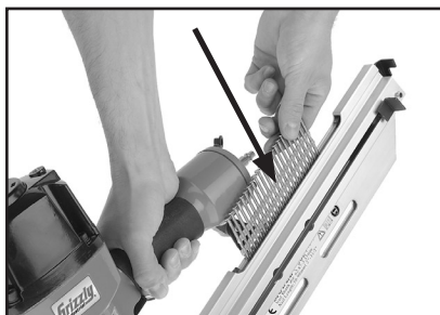
Figure 4. Loading nails into the magazine.
