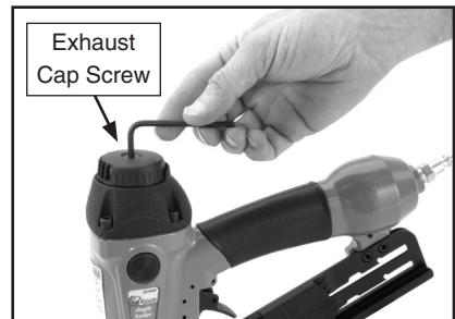
Figure 6. Loosening the exhaust cap screw.
