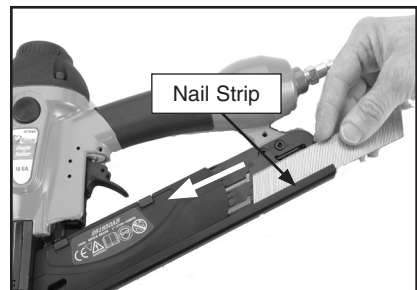
Figure 5. Loading a nail strip into the magazine.
