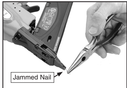
Figure 9. Using pliers to remove a jammed nail.
