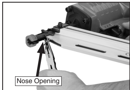
Figure 7. Nose opening for clearing jams.
