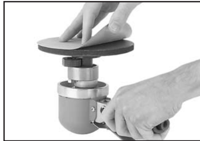
Figure 9. Attaching sanding disc.
