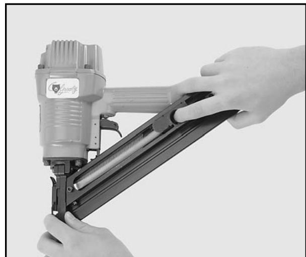
Figure 4 shows pulling back the spring handle to secure the nails and add pressure.
