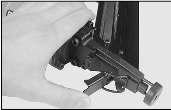
Figure 9 shows the safety clip that keeps the nose of the gun closed.
