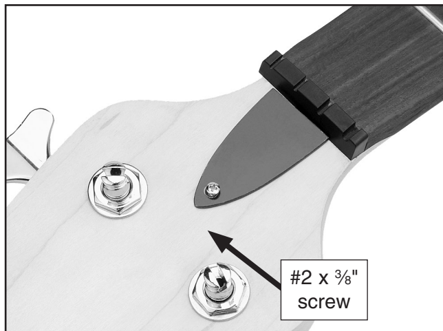
Figure 26. Truss rod cover installed.
