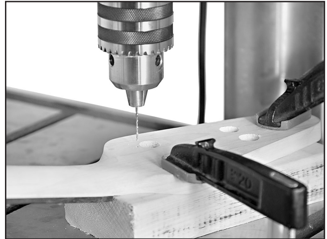
Figure 17. Drilling tuner mounting holes.
