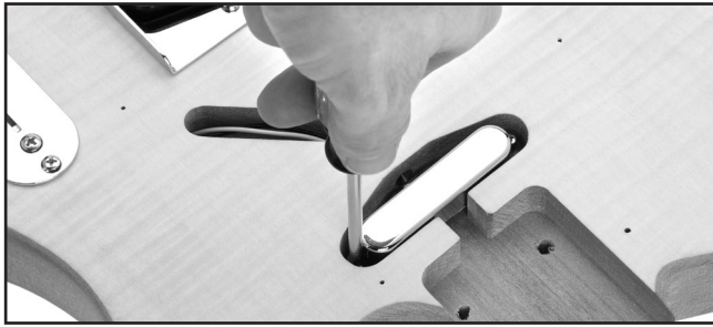
Figure 26. Fastening pick guard pickup.
