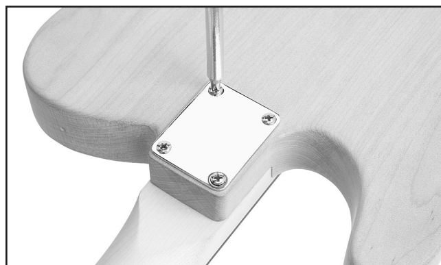
Figure 12. Fastening neck to body.
