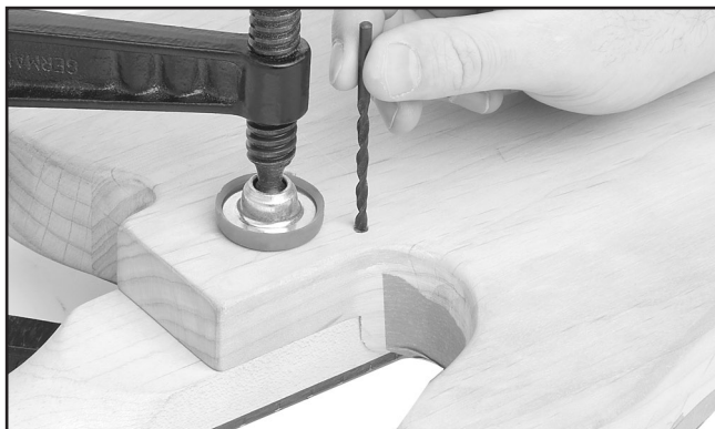
Figure 10. Making a pilot hole in the neck.
