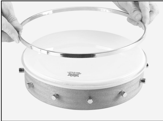
Figure 6. Installing the tension hoop.
