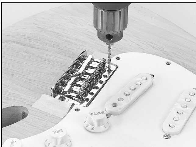
Figure 21. Drilling the bridge mounting holes.
