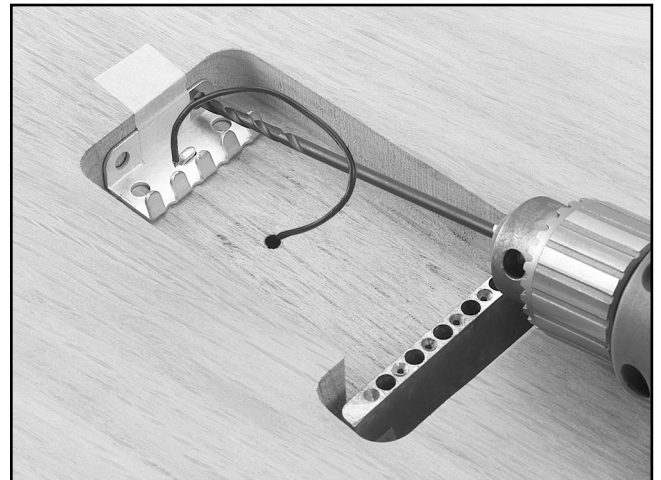
Figure 23. Drilling the spring hanger mounting holes.
