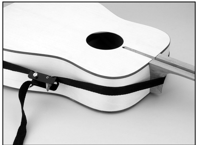
Figure 5. Clamping the neck/body assembly.
