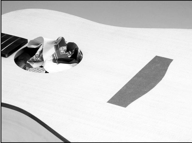
Figure 10. Masked bridge area and blocked sound hole.
