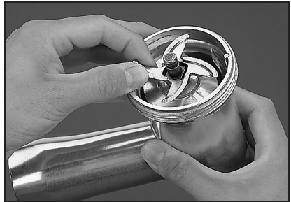
Figure 3. Cutting blade installation
