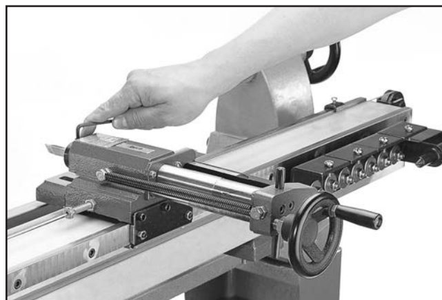
Figure 12. Securing cutting tool.
