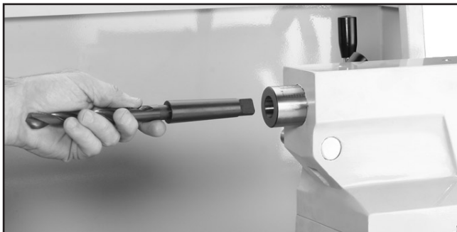
Figure 29. Example of drill bit installation.
