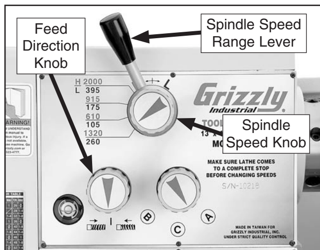
Figure 23. Headstock controls.
