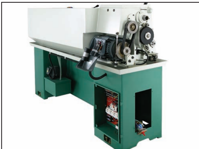
Figure 147. Electrical cabinet and motor wiring.
