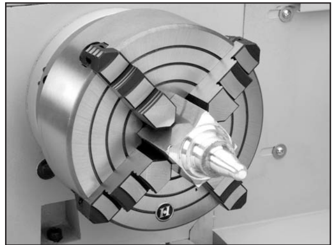
Figure 47. Generic picture of a workpiece properly mounted in a 4-jaw chuck.
