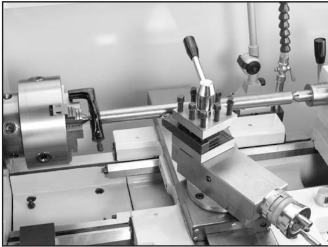
Figure 60. Generic picture of the test stock mounted between centers.
