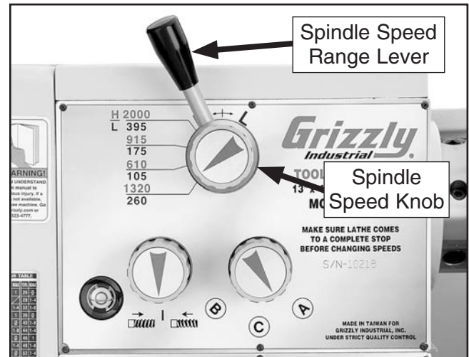
Figure 74. Controls used for setting the spindle speed.
