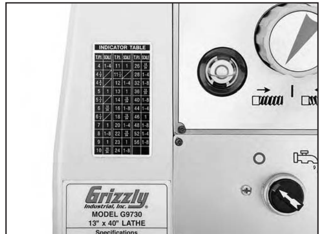
Figure 87. Thread indicator table.
