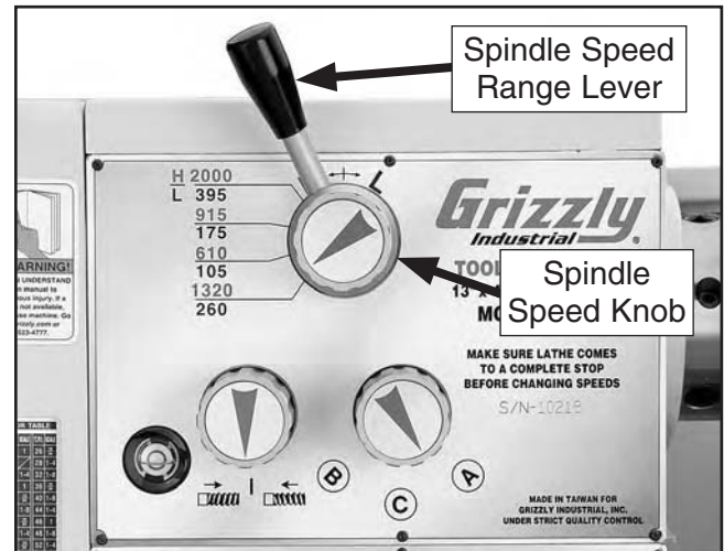
Figure 74. Controls used for setting the spindle speed.
