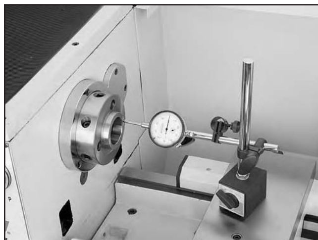
Figure 144. Example of preload dial indicator setup.
