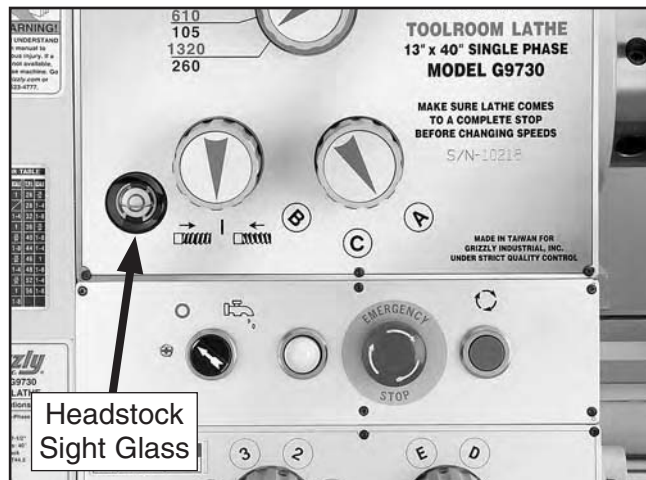
Figure 101. Location of headstock sight glass.
