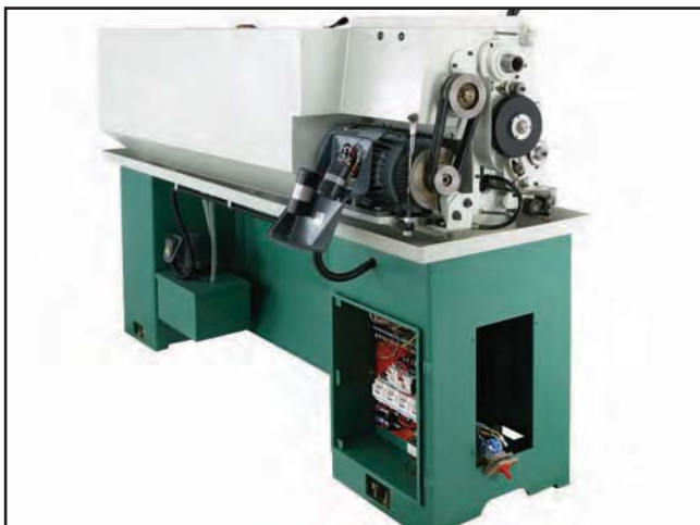
Figure 147. Electrical cabinet and motor wiring.
