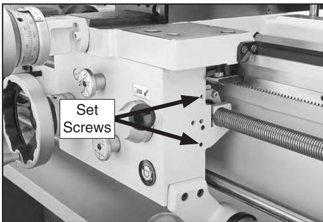
Figure 128. Halfnut gib set screws.
