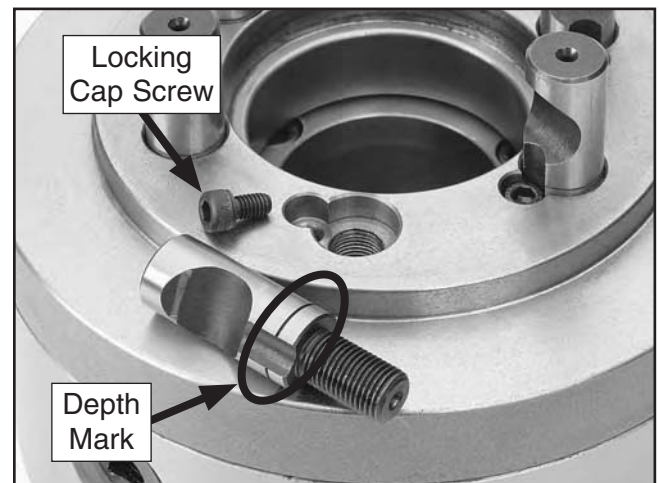
Figure 35. Camlock depth mark and locking cap screw.
