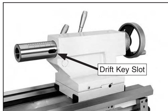
Figure 56. Location of the quill drift key slot.
