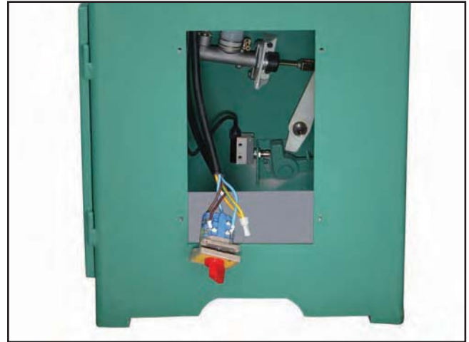
Figure 148. Main power switch wiring.
